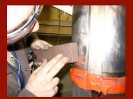
Skilled technicians hand dress the built up copper and blend with the shaft.
