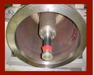
Grayloc seal area damage on FM housings is historically up to .007" in depth.
