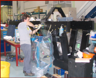
Brush Plating repair done on an oversized bearing fit on the FM frame unit.
