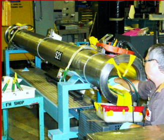
Score damage on I.D. of the RAM barrel housing being repaired with Brush Nickel Plating
